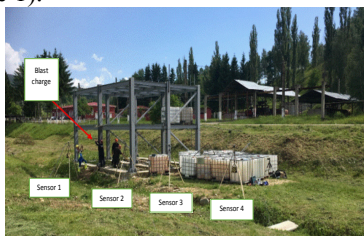
Figure 1. Testing setup, steel frame structure and location of overpressure sensors
